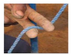
Turn your hand. If the turn can be completed between 90 and 180 degrees, the rope tension is ok.
