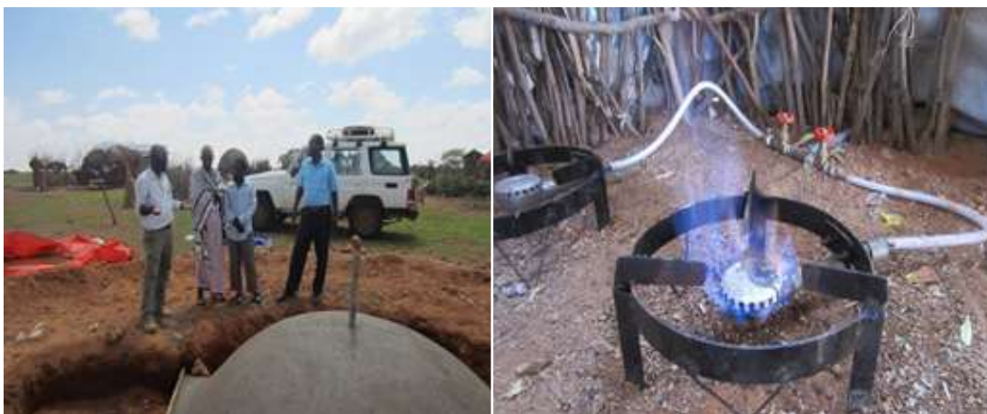
Figure 23: Biogas digester and strong flam from the biogas digester
