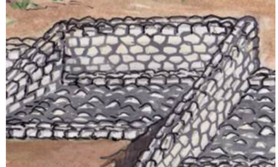
Figure 19: Constructed main wall of water spreading weir
