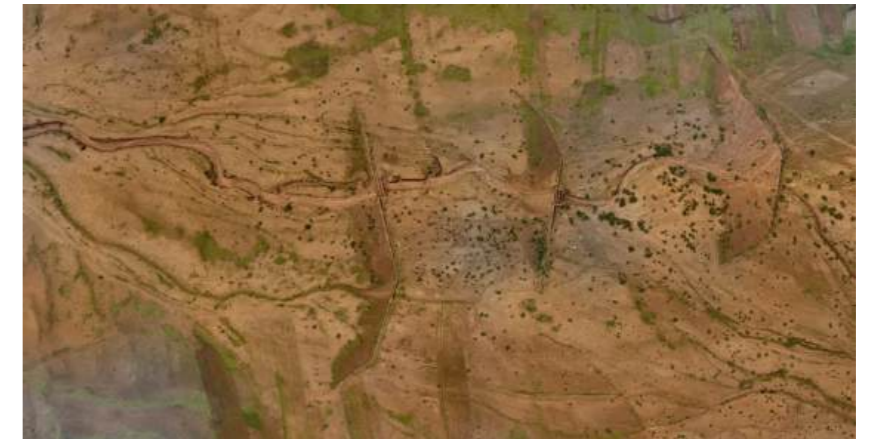
Aerial view of three WSWs built in cascades
