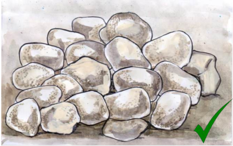
Use large stones for WSW construction.
