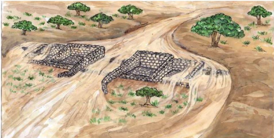
Figure 2: Illustration of Water Spreading Weir during floods
