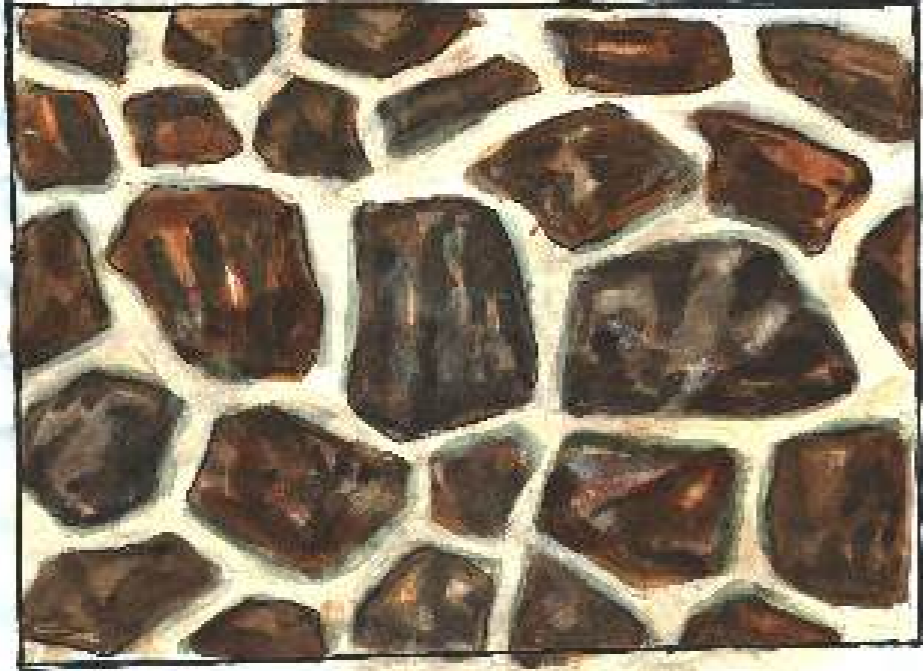
Figure 20: Detail of constructed wall showing the stone shape
