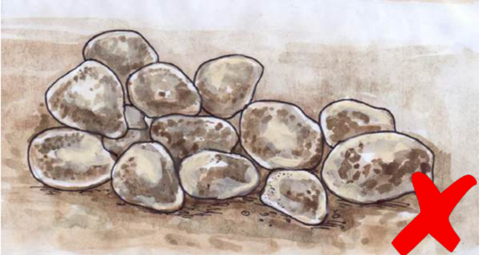
Never work with dirty stones – the weir will not be stable!
