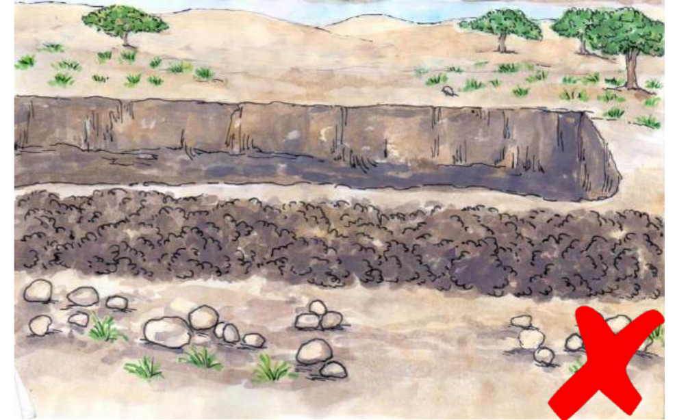
Never place the excavated soil on the downstream of the WSW during construction
