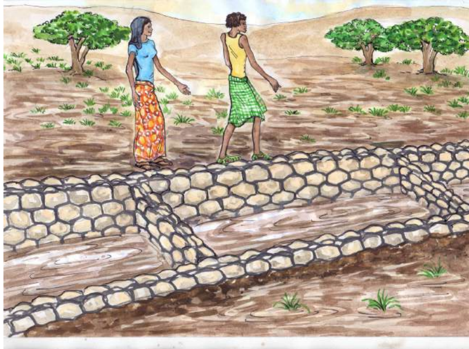
Figure 22: Counter wall and section division
