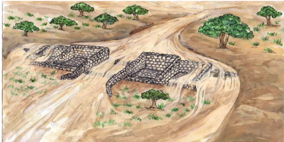
Figure 2: Illustration of Water Spreading Weir during floods
