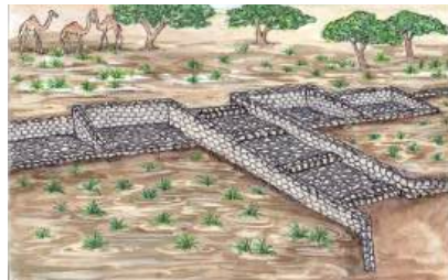
Figure 3: Water Spreading Weir along a dry stream in Afar
