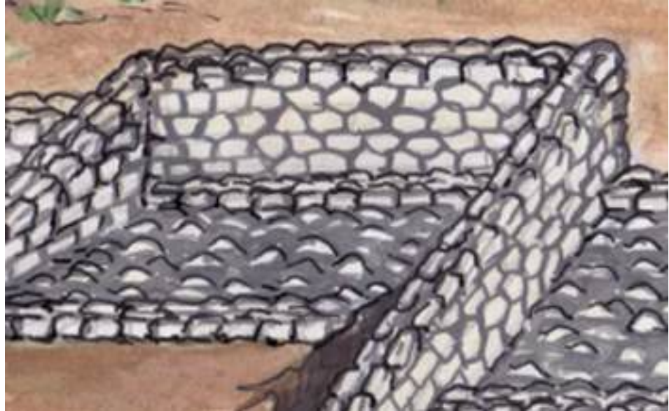
Figure 19: Constructed main wall of water spreading weir
