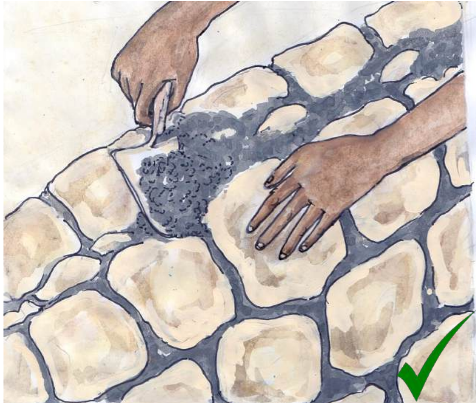
Making the stone and cement together at the same time.
