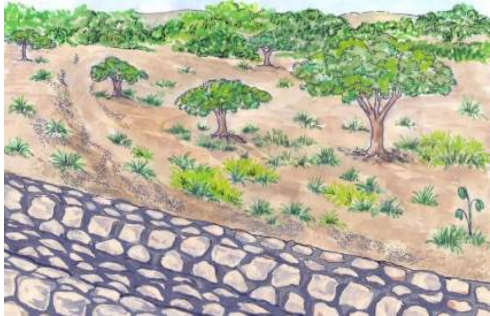
Figure 3: Absence of vegetation can lead to erosion, which can weaken the Water Spreading Weir structure
