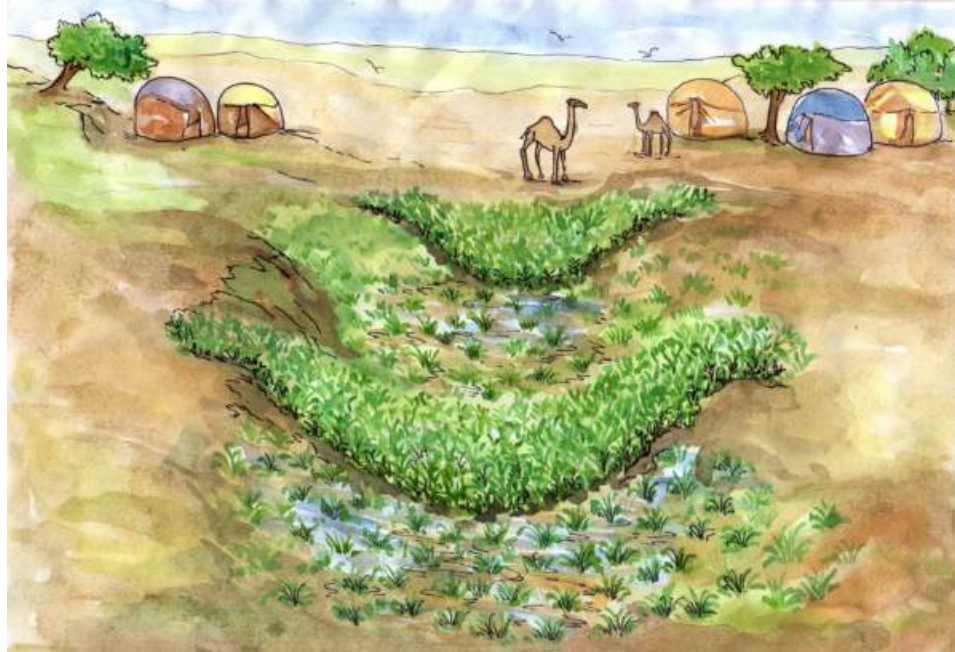
Figure 11: Biological check dams contributing to the stabilisation and restoration of gullies
