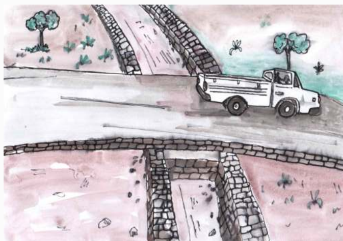
Picture 8: Soil over passage to allow vehicles to pass the structure.
