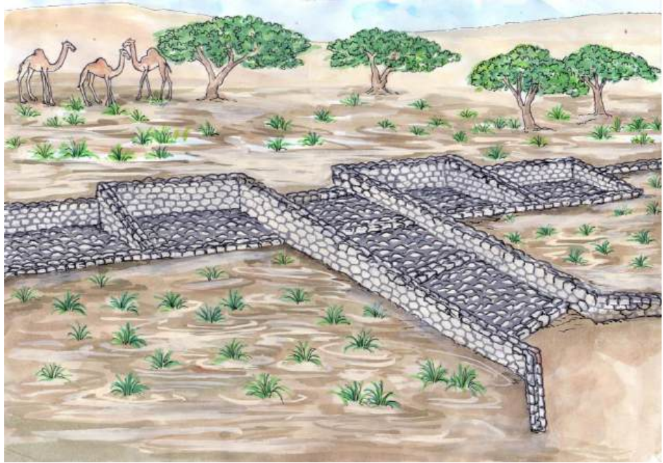
Illustration 18: restoration with a Water Spreading Weir
