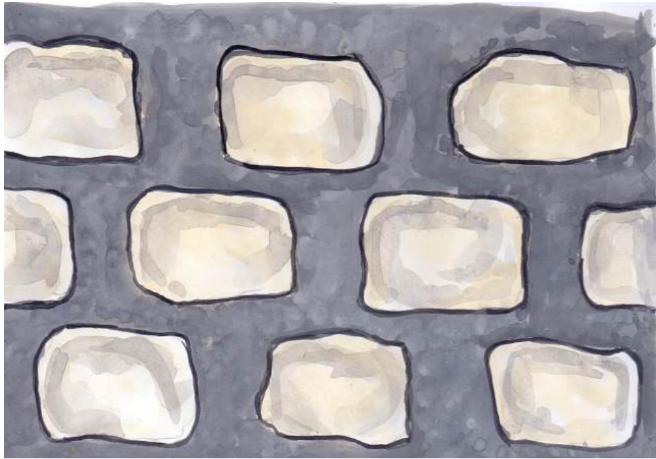
Illustration 34: Never lay stones loosely together or widely spaced apart: the weir will not be stable
