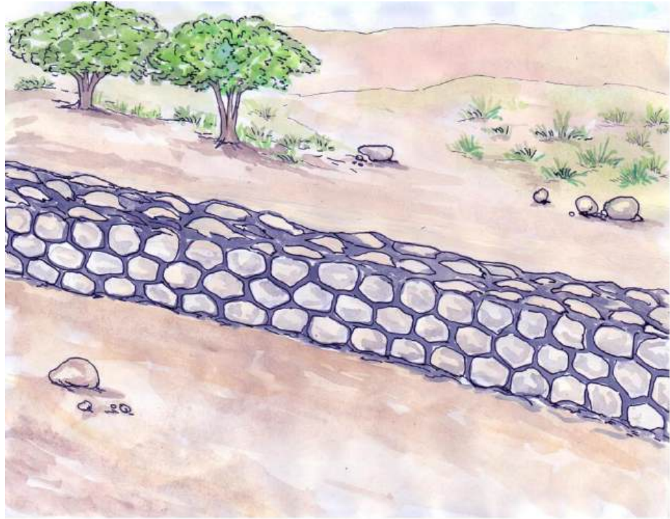
Illustration 40: Never build a straight long wall without buttresses: it will not be stable and will not last.
