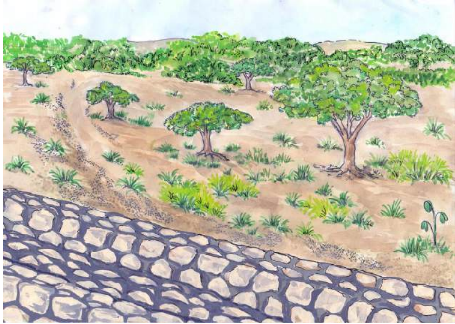
Illustration 6: The WSW causes temporary flooding and sedimentation above the main wall and along the wings
