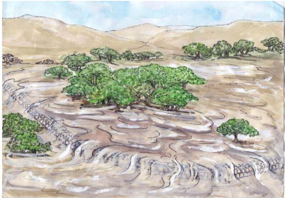
Illustration 8: A Water Spreading Weir is overflowed.
