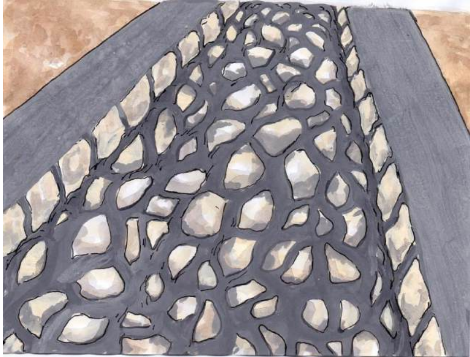
Illustration 38: Do not waste mortar making the surface smooth and flat. You are not building a garden or house wall and roughness will do more to slow water.
