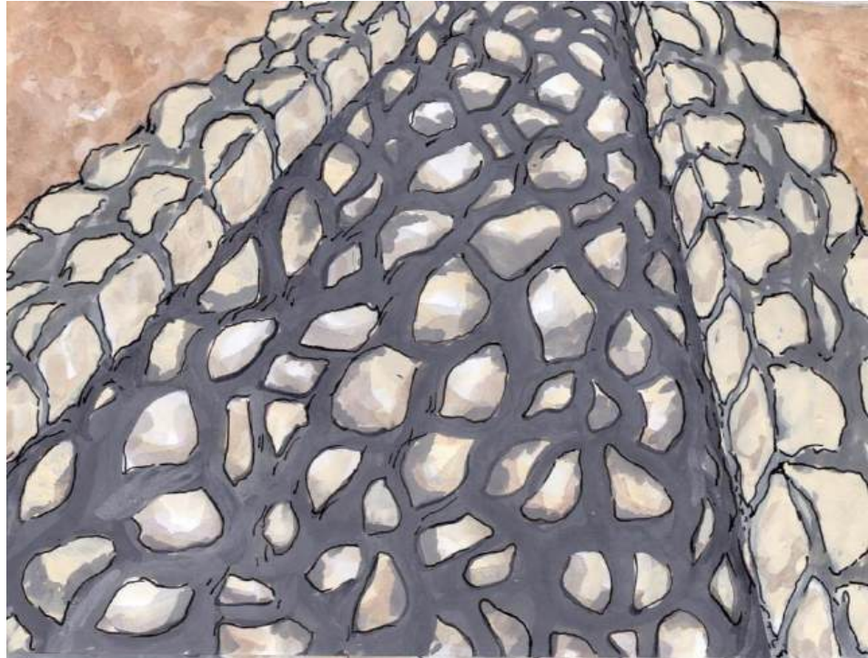
Illustration 37: Build a rough surface along the top of the weir: it is more effective at slowing down surface water
