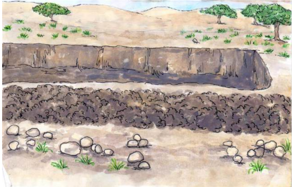
Illustration 42: Don't leave excavated soil downstream
