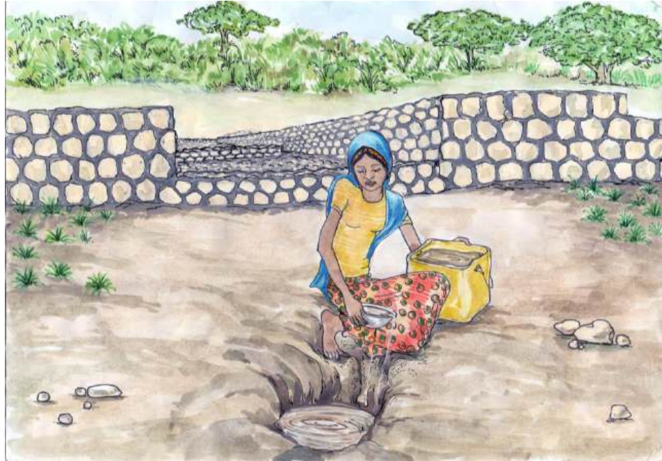
Illustration 12: Natural rehabilitation above the weir stabilizes the valley. Stored water below the surface eases the workload of women.
