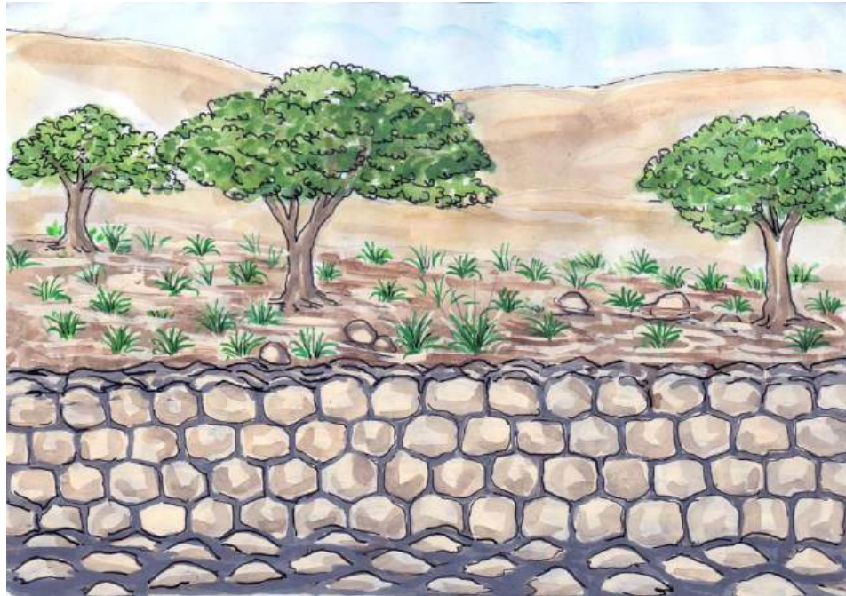
Illustration 9: Sedimentation after heavy rains above the wing of a Water Spreading Weir.
