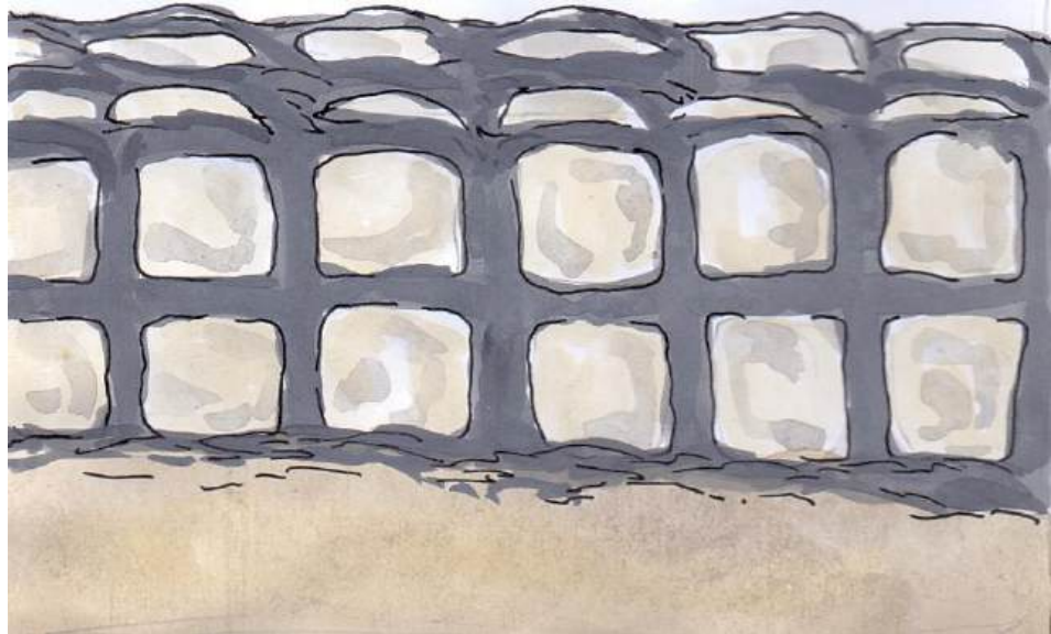
Illustration 36: Don't lay stones in vertical lines.
