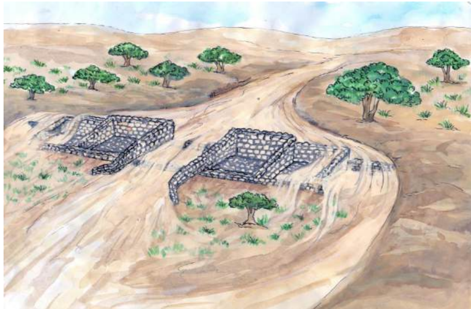
Illustration 5: a WSW spreads water and its sediment and reduces the velocity of water flow by enhancing the length of the water way
