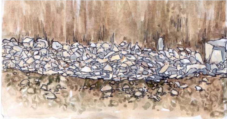
Illustration 32: Never lay mortar only! Mortar without stones is unstable and useless.
