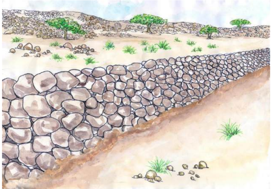
Illustration 21: finalized drystone structure
