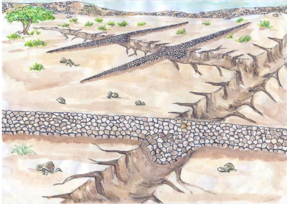
Illustration 4: Drystone structures can also be constructed within small gullies, but with a water spreading effect
