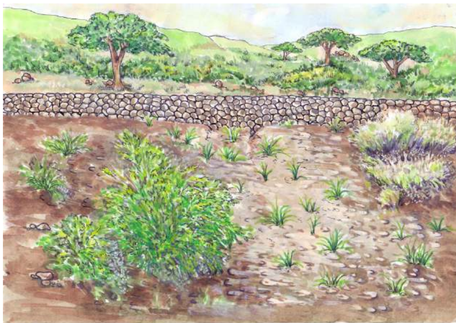
Illustration 30: Upstream of the drystone structure: fertile and moist soil with natural regeneration of grasses and shrubs
