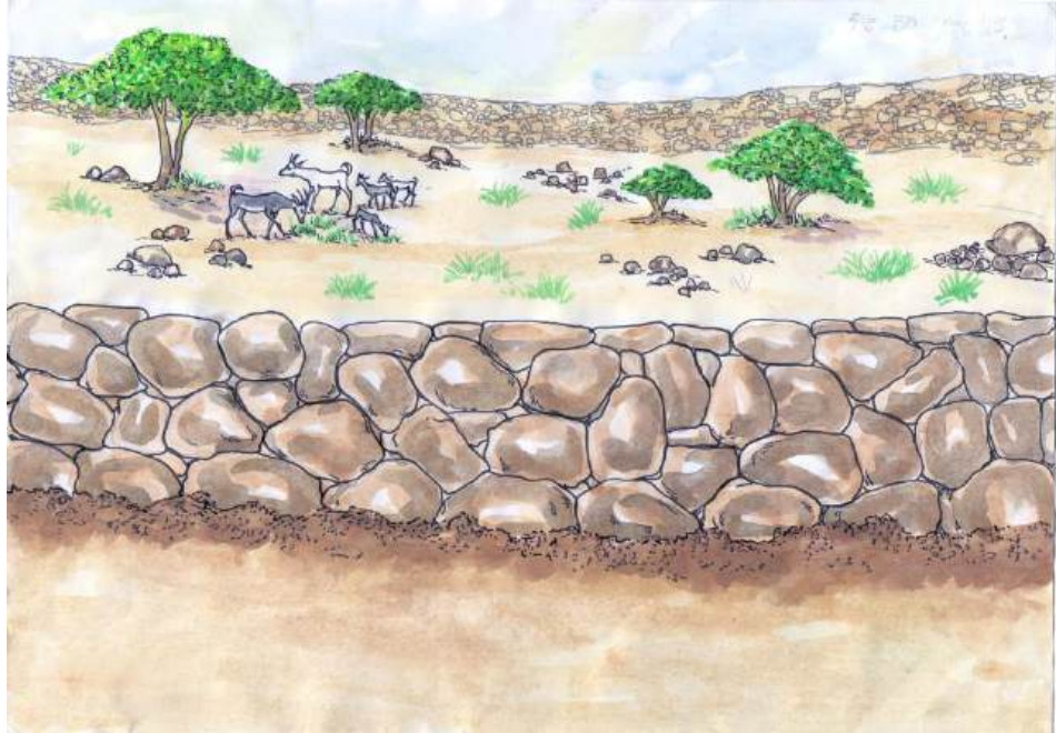
Illustration 26: Big stones are dug into the soil at the bottom line. The upper half of them is visible.
