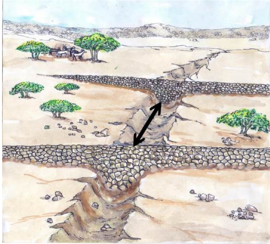
Illustration 11: Distance between dry-stone dams
