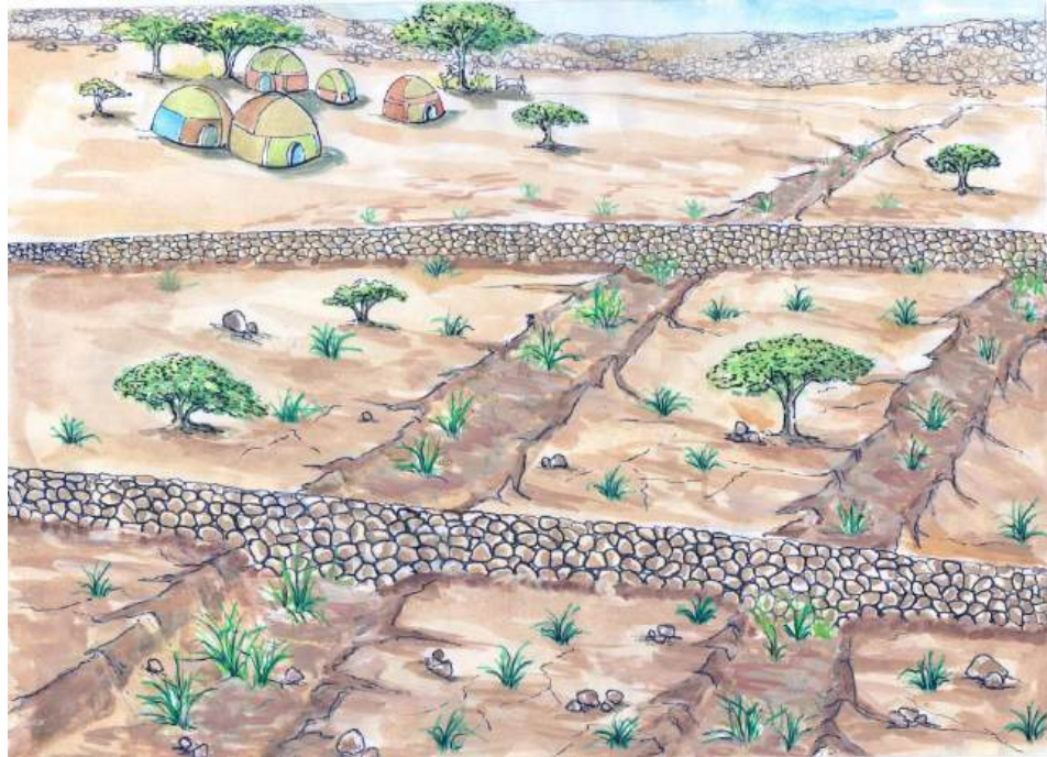
Illustration 5: Sequence of two dry-stone dams. Sediment and water infiltrate, enriching the land above and below the dry-stone dams
