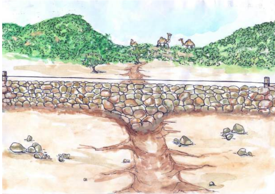
Illustration 14: A drystone structure is spanning the valley, forming a horizontal line. The width is increasing with the height of the structure, especially in the gullies
