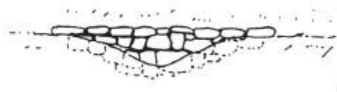
Figure 3: Level soil bund reinforcement at depression point
