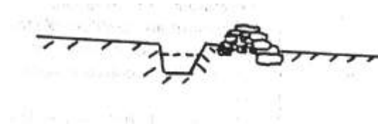
Figure 15: Integration of stone bunds with trenches
