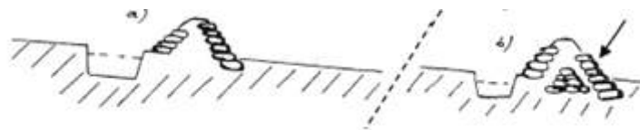
Figure 9: Double faced stone/soil bunds with collection trench
