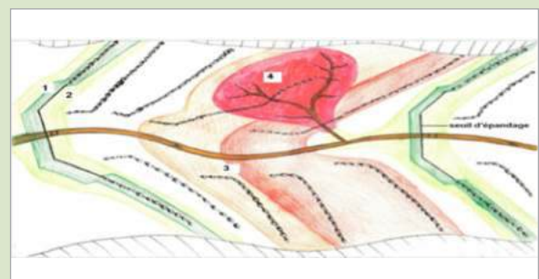
Figure 6: Areas above and below the weirs are well protected (1, 2); the risk increases in direct proportion to the distance from the upper weir (3) and gullies may form (4)
