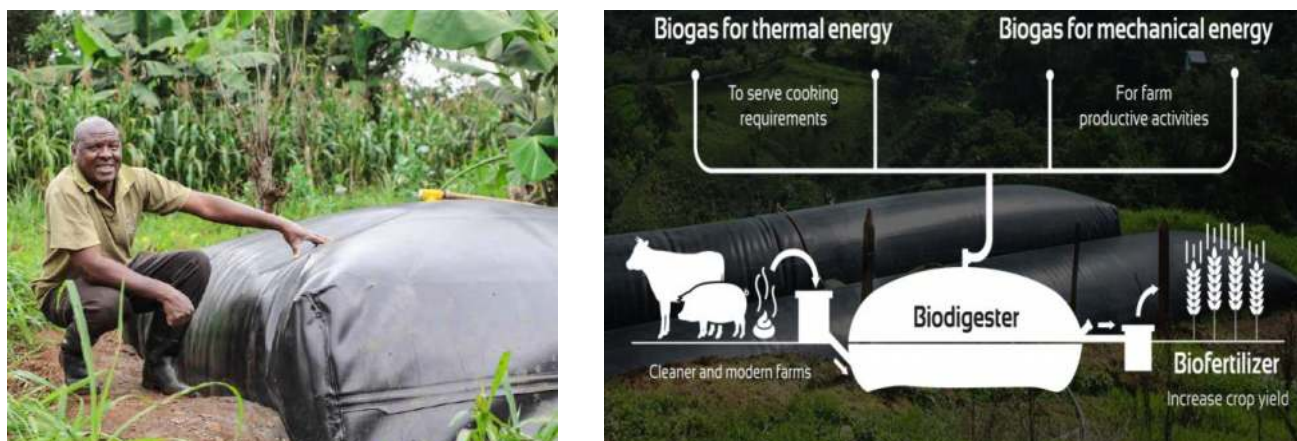
Figure 13: A small bio-digester and its components parts
